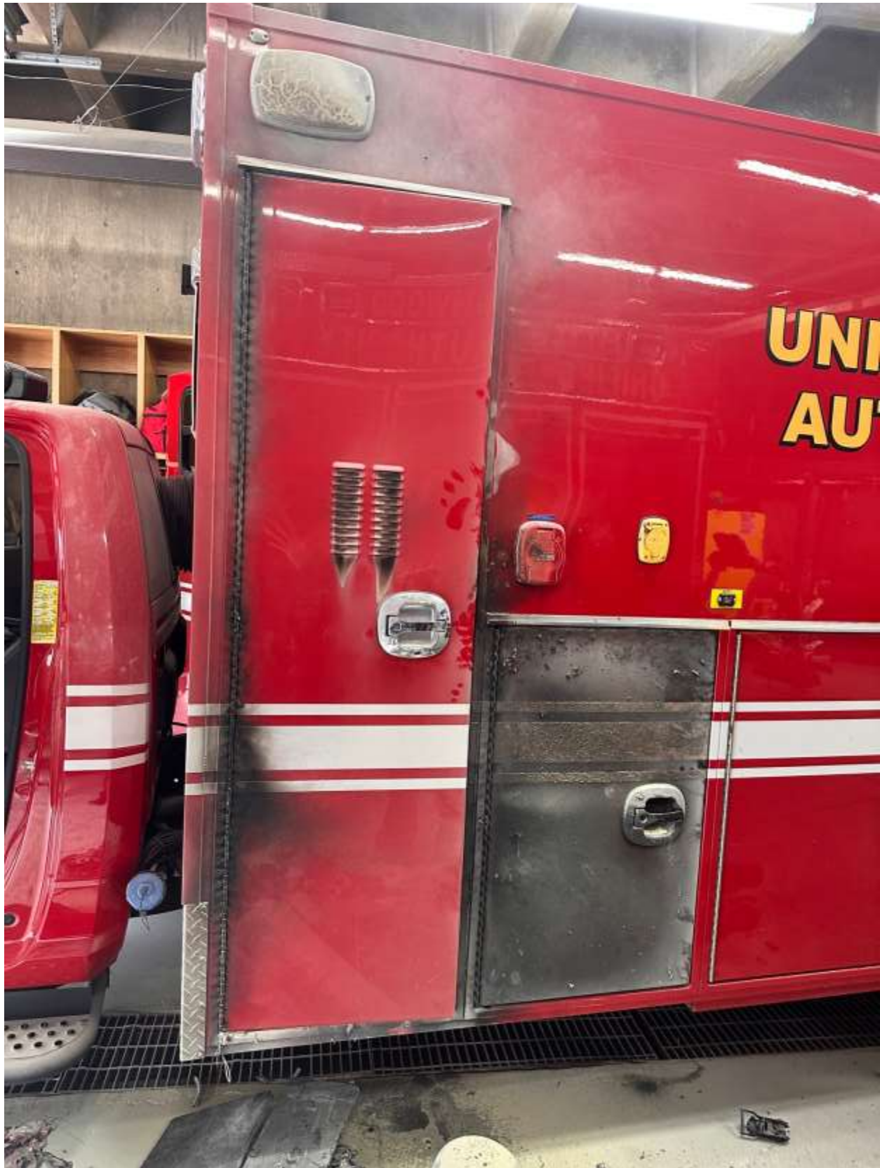
Image 10 – View of Damaged ME113 Compartments
