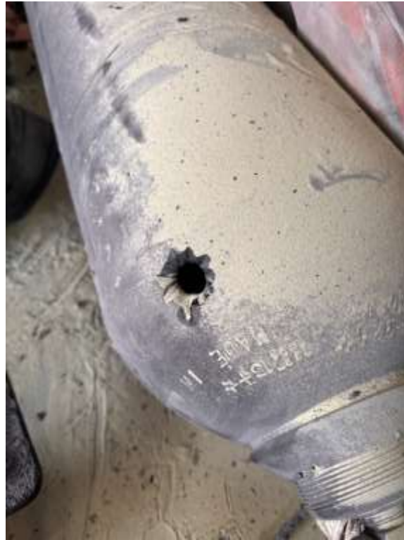
Image 8 – View of Damaged Oxygen Tank
