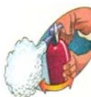
**S** **SWEEP.** Sweep from side to side at the base of the fire until it appears to be out. Watch the area. If the fire re-ignites, repeat steps 2 through 4.
