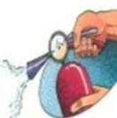
**S** **SQUEEZE.** Squeeze the handle to release the extinguishing agent.
